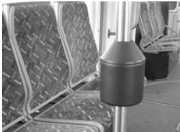
Figure 10. LF antenna mounted on a pole.
